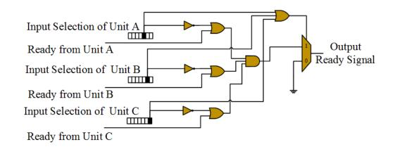
Suppose there are 3 units A,B,C. aCb - unit B is configured to receive data from unit A aR - ready signal from unit A Ra - ready signal to unit A
