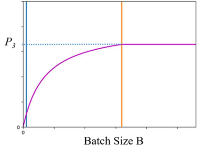
$$P = \frac{M_{op}B}{\frac{M_{op}B}{N_{pe}}} = N_{pe} \quad \text{when } B \geq \frac{N_{pe}}{N_t} \quad (2)$$
